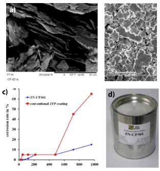
**Fig. 10a-d:** HKP-ZFP (Zinc-Flake by Simoloyer®), a) SEM), b) corresponding Zn-lamellar layer, c) corrosion rate of ZN-CP301 vs. conventional ZFP coating at salt spray test and d) a product can of anticorrosive paint ZN-CP301
