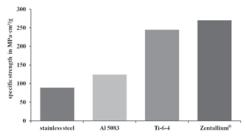
Fig. 5: specific strength of stainless steel, AI- and Ti- alloys and Zentallium®
