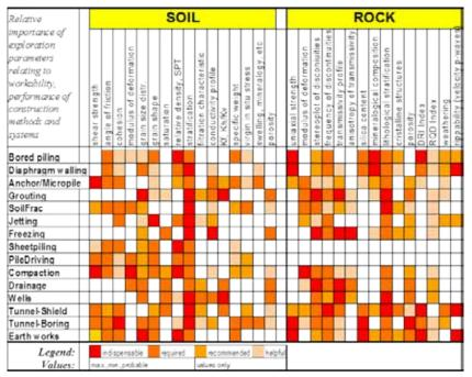
*Fig. 3:* »Qualitative significance of geotechnical parameters to be explored for different specialized foundation works«.
