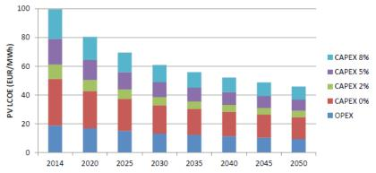
**Fig. 3:** PV LCOE evolution for a ground-mounted system in Munich, Germany for three different weighted average cost of capital (WACC) rates.
