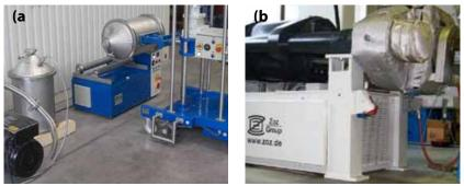
**Fig. 2a-b:** Passivation of Zentallium<sup>®</sup> powder after Simoloyer<sup>®</sup> – processing and hot extrusion at ZTC
