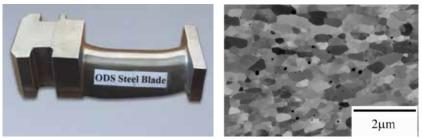
*Fig. 11:* turbine blade from ODS steel (picture taken from Zoz-ARCI Center, India) and BSE SEM image of 14 YWT (DiDomizio 2014)
