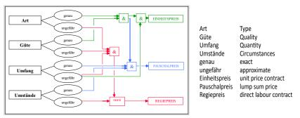
Fig. 1: »Recommendation in Austrian Standard ON A 2050 on how to relate type of compensation/contract to quality of description of the works.«
