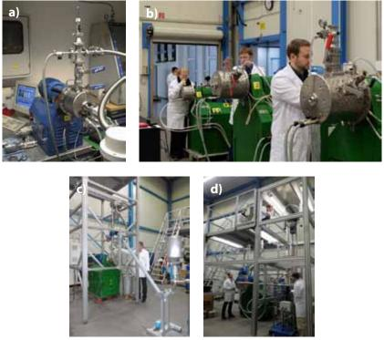
Fig. 1: a) Simoloyer® CM01-2Im laboratory scale with air-lock, b) Simoloyer® CM08Im (back) and CM20Im in front, c) Simoloyer® CM20-20Im-s1 semi continuous operation mode and d) Simoloyer® CM100-s2, auto-batch operation mode
