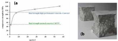
Fig. 6a-b: Compressive strength of FuturBeton vs. ordinary concrete (OPCC) and high performance concrete (HPC) and »used« ASTM test-cubes (b)
