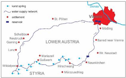
Fig. 4: Vienna is supplied with drinking water from karst springs nearly 200 km away via two long-distance mains (Source: Vienna's Water Supply, 2016).
